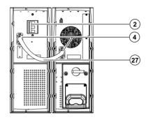
Connect cable (27) to the connectors (4) of the electronic and battery modules.
